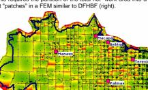
The introduction of continuity conditions along the patch borders analogue to the DFHBF implies restrictions between the transformation parameters d of neighbouring patches. Fig. below shows the patch-layout for the computation of the GIPS-1 databases between Sirgas and SAD69 and SAD96 Brazil. The regional transformation accuracies are in dark green (1 cm), bright green (5 cm), yellow (10 cm) and orange (20 cm).
